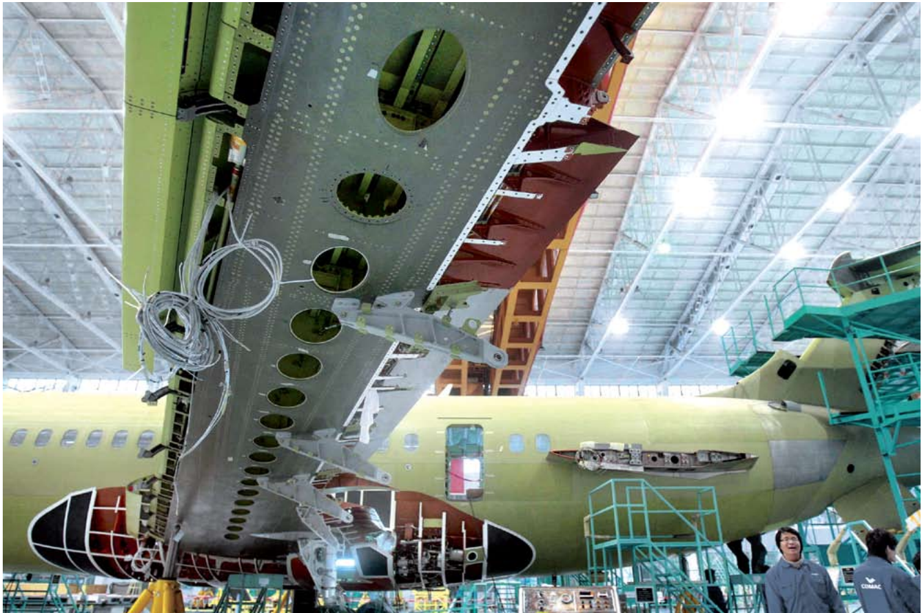
Montage eines Regional-Jets in der Shanghai Aircraft Manufacturing Factory in Shanghai.
